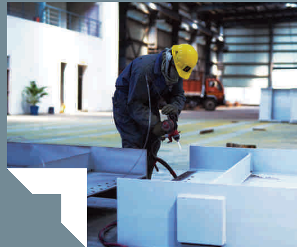
Al spray metallizing process
